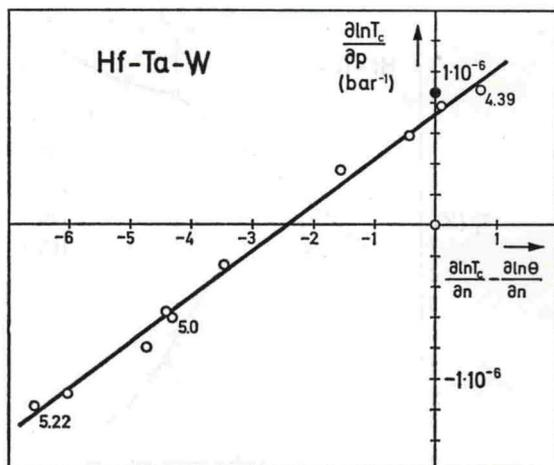
Fig. 2. Plot showing the linear relation between  $\partial \ln T_c / \partial p$  and  $\partial \ln \tau / \partial n$  for all alloys. The full circle represents  $\partial \ln \theta / \partial p$  for Ta
